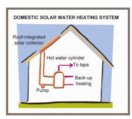
Active solar heating systems, including a solar collector on a south-facing roof, can contribute to heating needs.
