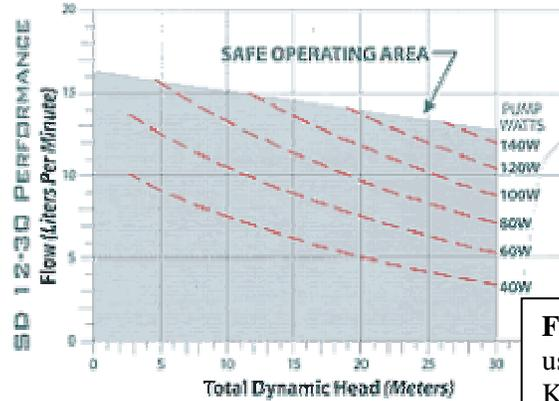
**Figure 8.** An example of a graph used to size a pump (from Kyocera Solar)
